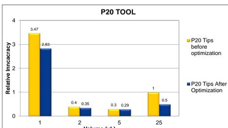
Figure 1. P20 Tool with P20 tips accuracy summary of before and after optimization.
