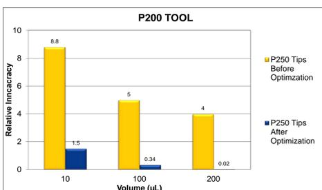
Figure 3. P200 Tool with P250 tips accuracy summary of before and after optimization.
