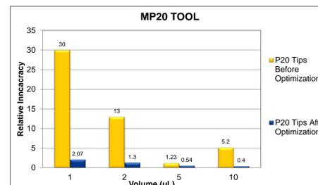
Figure 2. MP20 Tool with P20 tips accuracy summary of before and after optimization.
