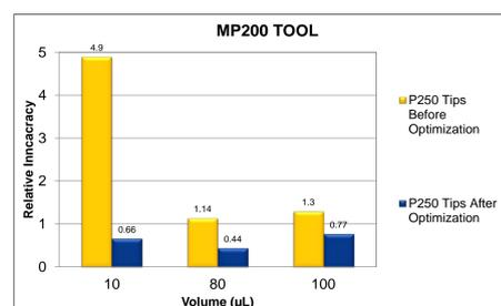
Figure 4. MP200 Tool with P250 tips accuracy summary of before and after optimization.
