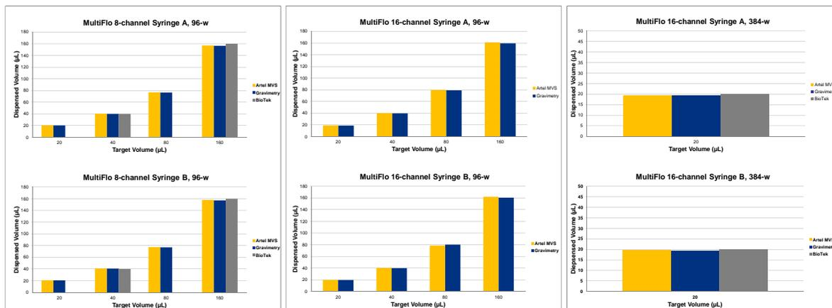
Figure 2. Overall averaged measured volume for: (top) 8-channel manifold with Syringe A into 96-w; (bottom) 8-channel manifold with Syringe B into 96-w.
