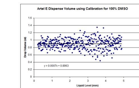
Figure 9 is data showing that the accuracy of the ATS-100 is insensitive to liquid height in the plate from which the droplet ejection occurs.
