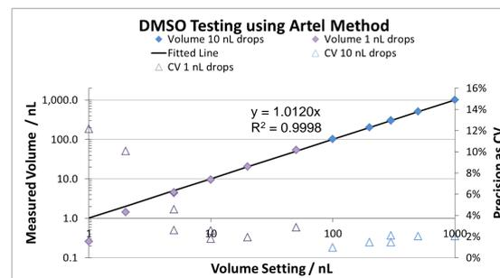
Figure 7: Accuracy and precision were confirmed to be excellent over the range of 10 to 1000 nL. At 1 nL and 2 nL the measurements show a departure from linearity which is attributed to the small absorbance signal obtained when using the Artel method far below the lower specified limit of 10 nL.
