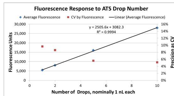
Figure 3: The average fluorescence response was linear over the range of 1 to 10 nL and show that ATS drop size is consistent and not dependent on dispense order. Precision data are plotted on the secondary axis.
