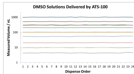
Figure 6: DMSO based MVS measurement results for each well are displayed in sparkline format. Data collected at volume settings from 5 nL to 1000 nL are shown in this figure.
