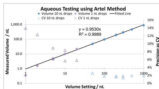
Figure 5: The MVS method delivers traceable results at 10 nL and above that the two systems (MVS and ATS-100) exhibited good co-linearity over the range of 10 nL to 1000 nL. ATS-100 data with droplet sizes of 1 nL and 10 nL are included in this figure.
