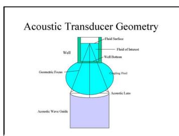
Figure 1: Acoustic energy is focused on the fluid surface to eject a droplet.
