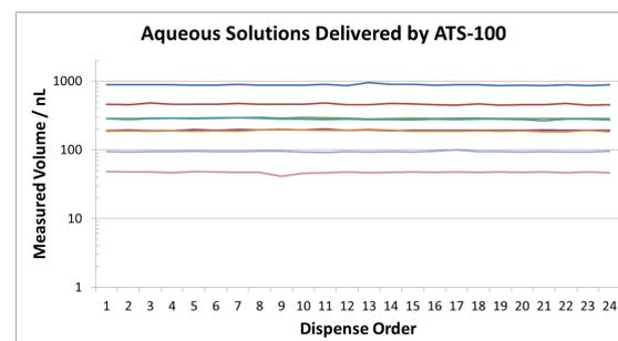
Figure 4: Aqueous MVS measurement results for each well are displayed in sparkline format. Data collected at volume settings from 50 nL to 1000 nL are displayed in this figure.
