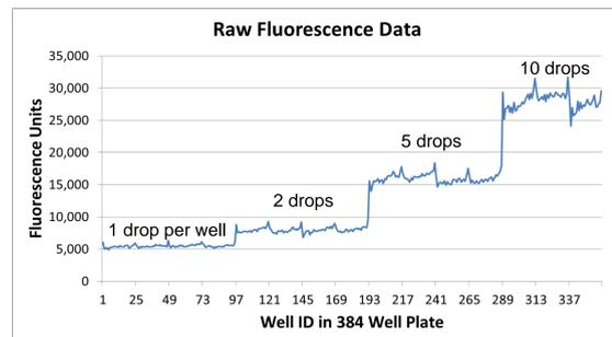
Figure 2: Raw fluorescence data are presented in sparkline format. ATS-100 droplet size was set to 1 nL and counts were varied from 1 to 10 drops per well. Some edge effect patterning was seen and is attributed to the fluorescence measurement method.
