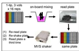
Figure 3. A Biomek 3000 with P20 head was used to transfer 16 reps of three different target volumes into a 96-well plate (wet-dispense). After each dispense, three "common" aspirate/dispense cycles were used to mix each well. When the 48 wells were completed, the plate was measured using the MVS. The same plate was then shaken using the MVS shaker before re-reading a second time. Finally, the plate was re-shaken on the MVS shaker and read in the plate reader for a third time.
