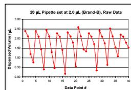
**Figure 1.** A 20  $\mu$ L pipette, set at 2.0  $\mu$ L, was employed to successively deliver reagents at temperature intervals of: 4 °C, 22 °C, 37 °C, 60 °C. Ten replicates of this interval were performed.
