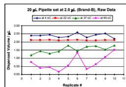
**Figure 2.** Data of Figure 1 were re-plotted to show the dispensed volume as a function of sample temperature.
