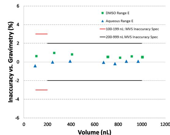
Table 1. MVS System Performance Specifications for Range E Sample Solution in 96-well Verification Plates
