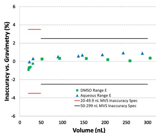
Figure 3. MVS Performance at 100-999 nL in 96-well MVS Verification Plates.
