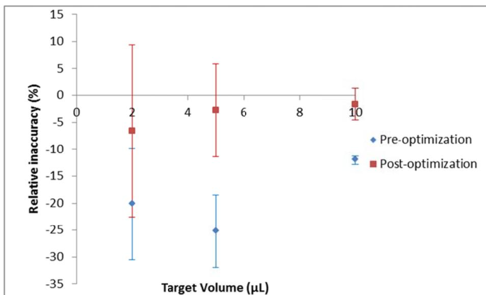
**Figure 2.** Pipetting performance data for 2, 5, and 10  $\mu\text{L}$  delivered by the Biomek 3000 using a P200L tool with P250 tips.
