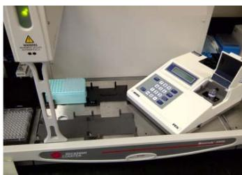
The PCS was placed directly onto the deck of the Biomek 3000 at an angle to allow optimal clearance for access by the robot. A 'labware' description of the PCS was created within the Biomek software. This
