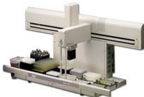
The Biomek 3000 is an automated liquid handler that incorporates various pipetting tools for common pipetting tasks, including single- and multi-channel pipetting heads.
