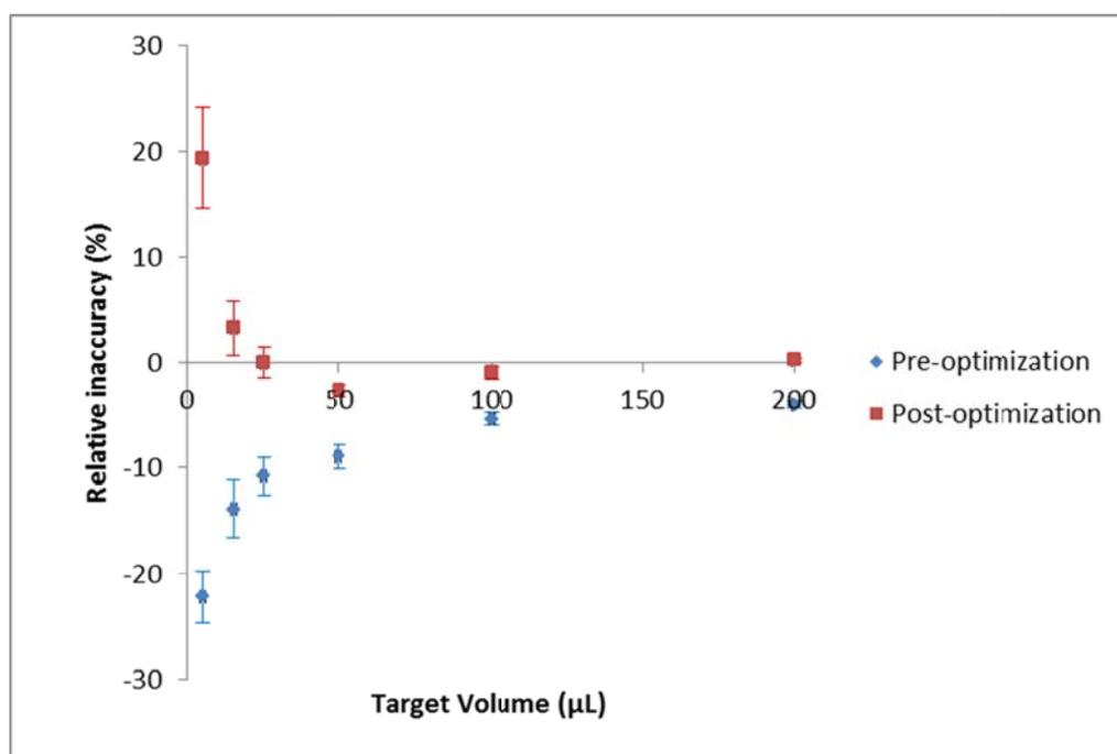
**Figure 1.** Pipetting performance data for volumes delivered by the Biomek 3000 using a P200L tool with P250 tips.
