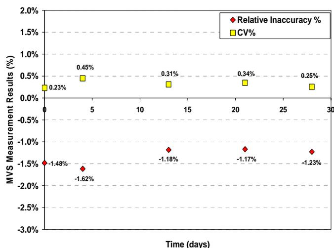
**Figure 5.** Using an 8- $\mu$ L calibrated syringe, the 19.34% glycerol test solution was verified on five different days over a 28-day period. Based on the relative inaccuracy values, the shelf-life of the solution may be at least 4 weeks.
